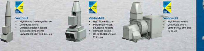
High Plume Dilution - Fan design that entrains and mixes outside ambient air into the exhaust airstream prior to exiting out the windband discharge. Potentially hazardous exhaust or exhaust fumes are diluted and dispersed quickly.
