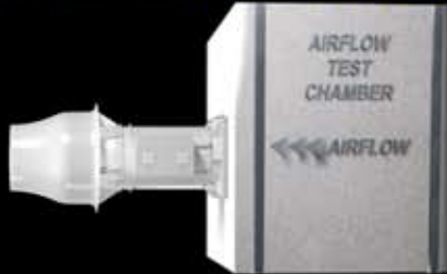
Setup #1 ( AMCA Standard 210, Figure 15 )
