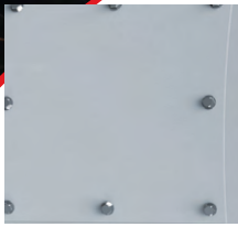
Bolted Inspection Door
