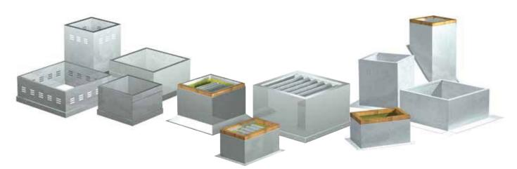
Prefabricated roof curbs reduce installation time and costs by ensuring compatibility between the fan, curb and roof opening. A wide variety of roof curbs are available including: flanged, straight-sided, canted, pitched, ridged, vented, and sound-absorbing. Extensions raise the fan discharge and can provide an accessible mounting location for dampers. Insect screen bases and vented extensions are also available.
