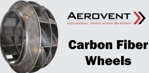
Aerovent's BCF fan is available with carbon fiber wheel in lieu of traditional fiberglass. Designated by the fan class (CF = carbon fiber; FG = fiberglass), the material change allows the BCF to reach RPM limits well beyond the limits of the traditional fiberglass. This higher limit translates into a fan able to reach pressures up to 34" w.g.
