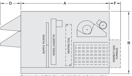
Drawings show both heating coil and indirect gas furnace options. Electric heat is also available. Only one can be selected.
