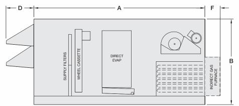
Drawings show optional indirect gas furnace. Electric heat is also available. Only one can be selected.
