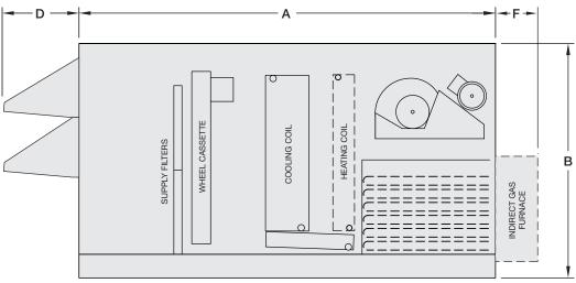
Drawings show both heating coil and indirect gas furnace options. Only one can be selected.
