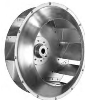
CPV uses a riveted aluminum wheel, with backward inclined flat blades.
